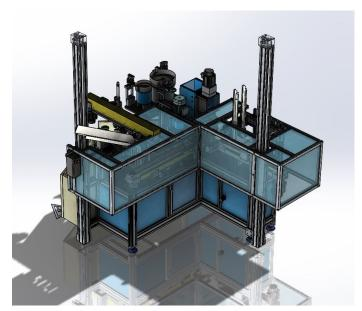
Nailing machine up to six nails with double vibrating station. Nails control system with six sensors. Nailing system, clamp closure and handle loader with servomotor.
